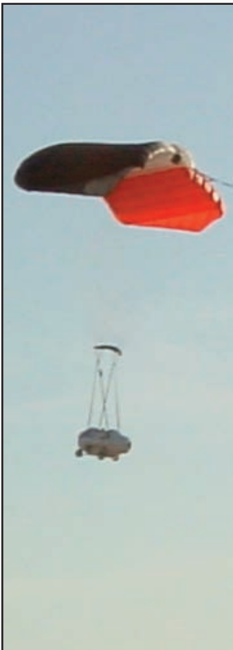
Nova 2 capsule parachute test
